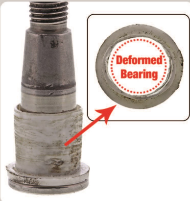
Plastic Bearing Design Continuous off-centre loading leads to deformation
